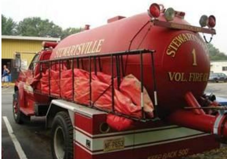
(1) Commercial tank vehicles that are converted for fire department use can easily become overloaded and dangerous. This unit was initially designed to haul liquid propane. (Photos by author unless otherwise noted.)
