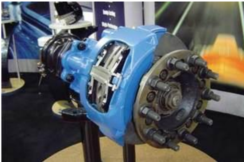
(3) Large disc brakes run cooler, stop better, and reduce brake fade.
