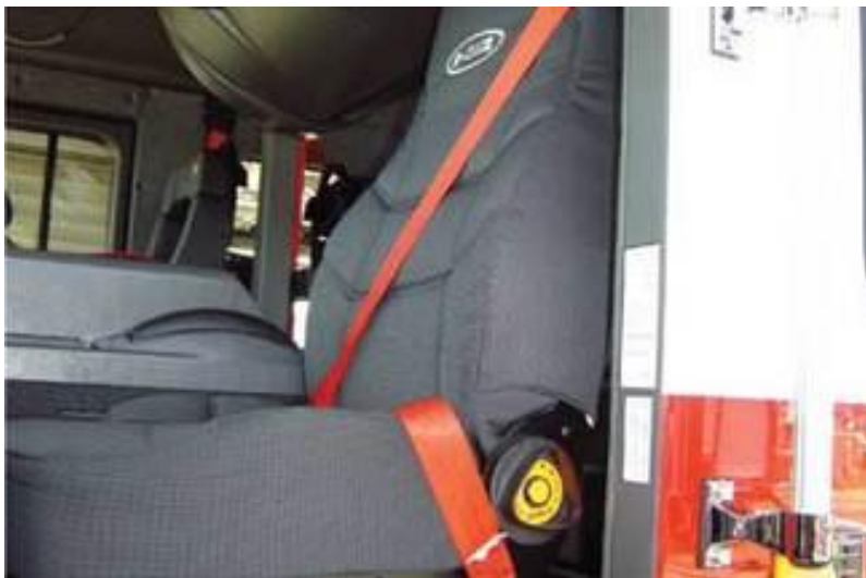
(2) Red seat belts for better visibility and stalks to make attachment easier were required in 1999.
