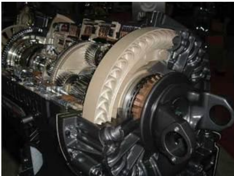
(4) The cutaway view of a hydraulic transmission retarder shows a large-fluted disc that is slowed down when the chamber fills with transmission fluid on activation.
