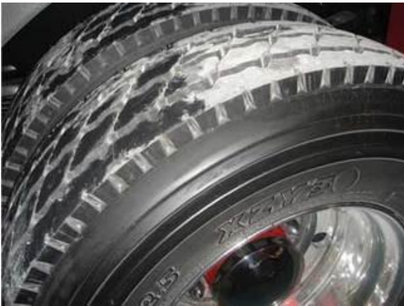
(6) The pattern of a tire's tread moves water out from under the tire. Properly inflated tires are extremely important in rollover prevention.
