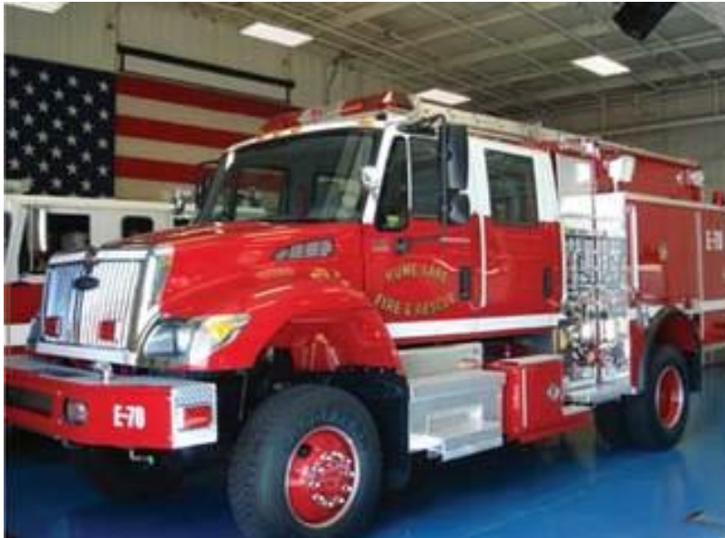
(5) The higher ground clearance on four-wheel-drive apparatus raises the center of gravity.
